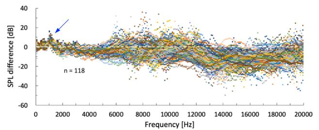
Fig. 2. Difference spectrum, subtracting sound pressure level (SPL) for HRTF for front direction from that for rear direction for 118 ears.
