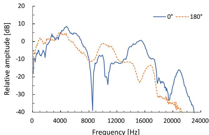
Fig. 1. Examples of HRTF for rear (180°) and front (0°) directions.
