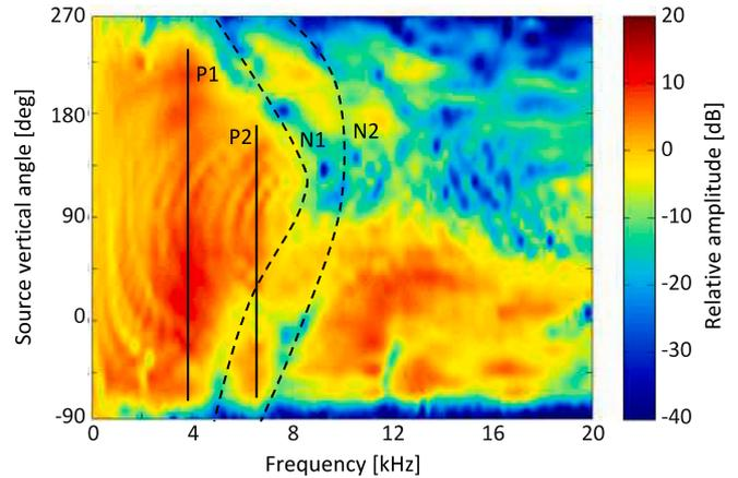
Fig. 6. Relationship between vertical angle of sound source and N1, N2, P1, and P2 frequencies in HRTFs in the median plane.
