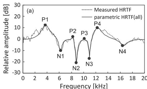
Fig. 5. Examples of parametric HRTFs [26]. (a) measured and parametric HRTFs with all notches and peaks, (b) parametric HRTF reconstructed using N1, N2, P1, and P2.
