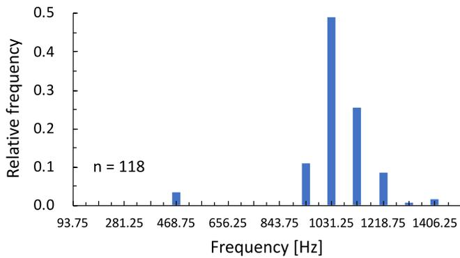
Fig. 4. Normalized histogram of frequencies for which SPL difference between rear and front HRTFs is maximum.
