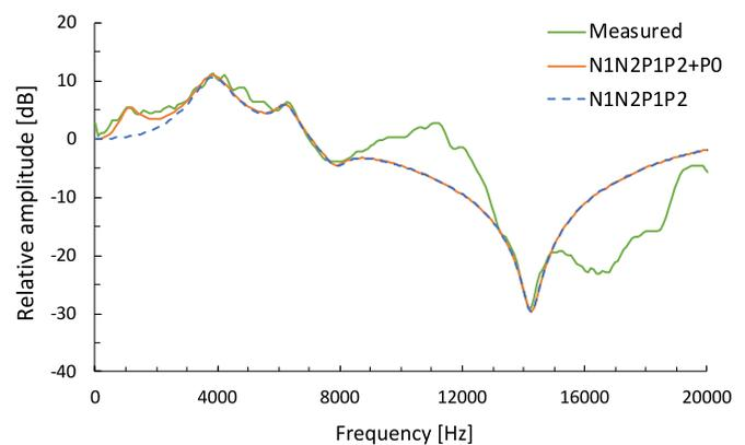
**Fig. 11.** Examples of measured HRTF and generated parametric HRTFs (N1N2P1P2 and N1N2P1P2 + P0) for rear direction.
