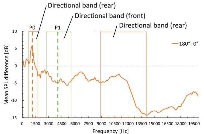
Fig. 7. Relationship between mean SPL difference between rear and front HRTFs for 118 ears (orange solid line) and directional bands for rear (orange outline) and front (green outline). The orange and green dashed lines indicate the mean P0 and P1 frequencies, respectively, averaged over 118 ears.
