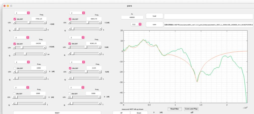
**Fig. 10.** Custom-made software for generating parametric HRTFs. The left side of the panel shows parameter settings for eight IIR filters, each of which creates a notch or a peak.
