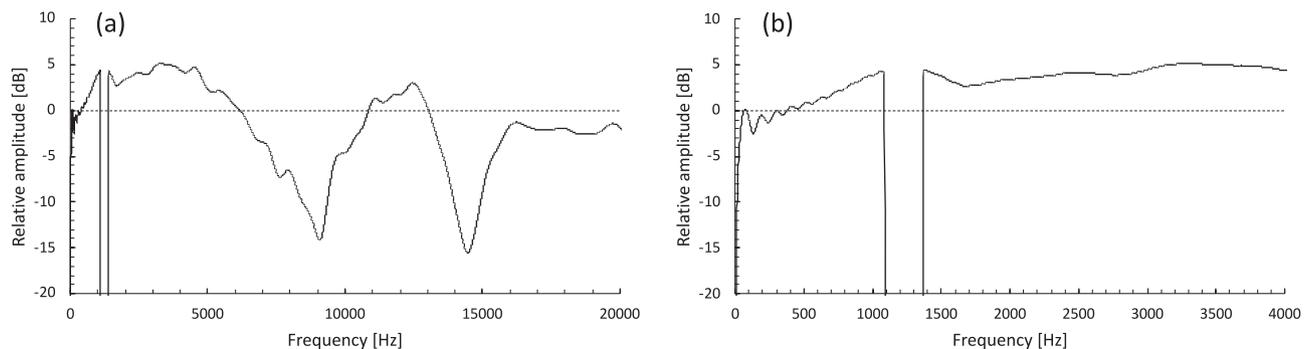
Fig. 8. Example of transfer function obtained by convolution of subject's HRIR at 180° and P0-eliminated filter. (a): 0–20 kHz, (b): 0–4 kHz.
