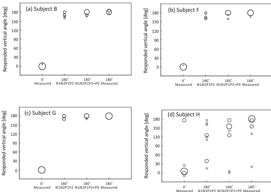
Fig. 12. Responses to measured HRTF, N1N2P1P2, and N1N2P1P2 + P0 for front and rear directions.
